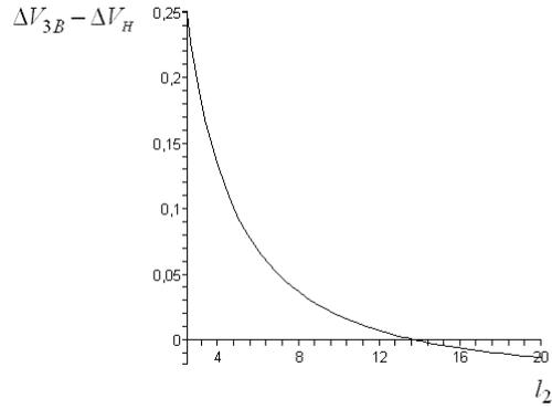
**Figure 11. The Difference of Characteristic Velocity (In Non-Dimensional Values). For the Three Burn Bi-Elliptical and Hohmann's Transfer As Function of  $l_2$  for  $l_1 = 1$ ,  $\alpha = 1 + l_2$**
