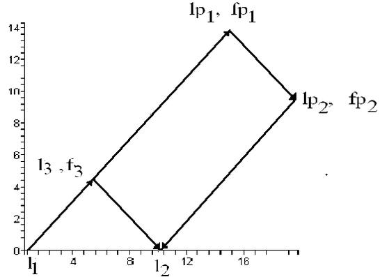
**Figure 9.** The Three Burn Bi-Elliptical Transfer From the Circular Orbit With Radius  $l_1$  To the Circular Orbit With Radius  $l_2$  and the Hohmann's Transfer. Hohmann's Transfer Corresponds To the Broken Line Including the Points:  $(l_1, 0) \rightarrow (l_3, f_3) \rightarrow (l_2, 0)$ . The Three Burn Bi-Elliptical Transfer Corresponds To the Broken Line Including the Points:  $(l_1, 0) \rightarrow (l_{p1}, f_{p1}) \rightarrow (l_{p2}, f_{p2}) \rightarrow (l_2, 0)$ .
