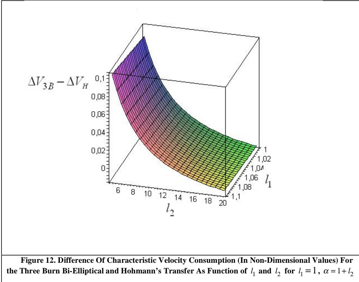
Figure 12. presents the difference in the characteristic velocity for the three burn and Hohmann's transfers for  $1 \leq l_1 \leq 1.1, 5 \leq l_2 \leq 20, \alpha = l_1 + l_2$ .
