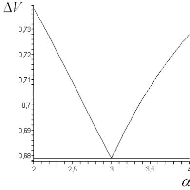
**Figure 10. Comparing The Characteristic Velocity For the Three Burn Bi-Elliptical and Hohmann's Transfer For the Radii of 1 And 3 For Initial and The Target Orbit Respectively. The Abscissa Axis Presents  $\alpha$  - The Ratio Of the Pericenter Distance of the First Transfer Orbit To the Radius of the Initial Orbit. The Ordinate Axis Presents the Characteristic Velocity Consumption In Non-Dimensional Characteristic Velocity Consumption For the Hohmann's Transfer.**
